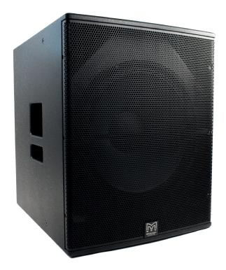
The X118 is a compact, high performance subwoofer for use with BlacklineX Series full-range loudspeakers. It extends the low frequency operating range of the combined system to 42Hz and provides exceptional low frequency impact. It can be used singly, stacked or flown via integral M10 insets and features a long-excursion 18" (460mm)/4" (100mm) voice coil driver in a compact reflex enclosure. Its four reflex ports have a large frontal area to reduce turbulent air noise at very high levels.
